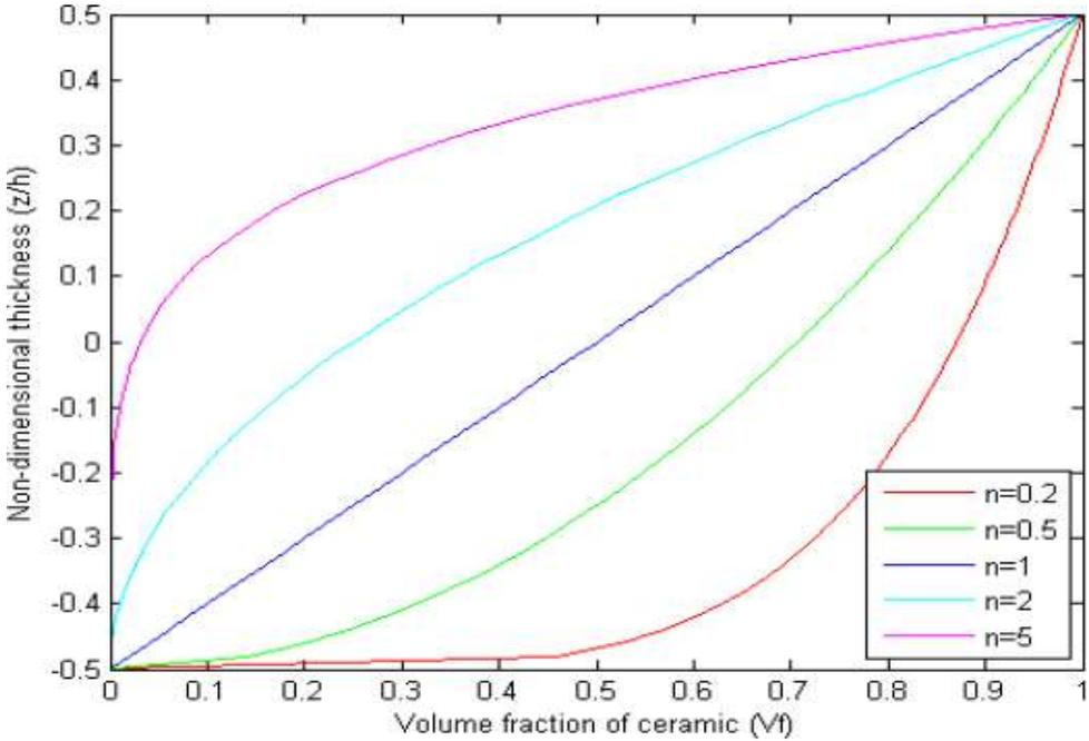
Figure 4.1 Shows The Variation Of  $V_f$  Through The Plate Thickness.
