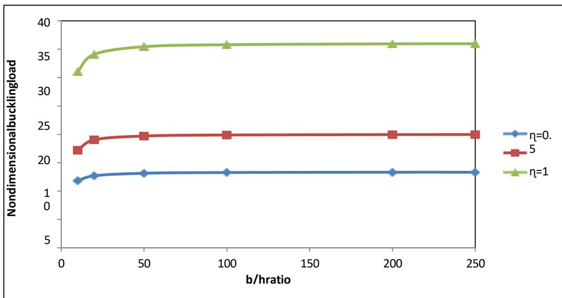
**Figure 4.4: Variation of non-dimensional buckling load with b/h ratio and load parameter ( $\eta$ )for SSSS plate and a/b =1**
