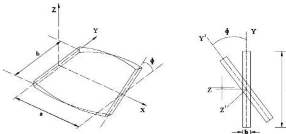
Figure 3.1: FGM twisted plate
