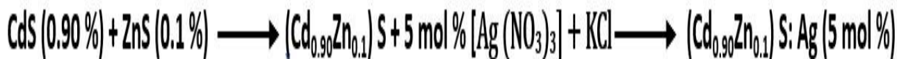
Figure 1. Mechanism of the solid-state synthesis of Ag (5 mol %)-doped (Cd 0.90 Zn 0.1 ) S phosphor.
