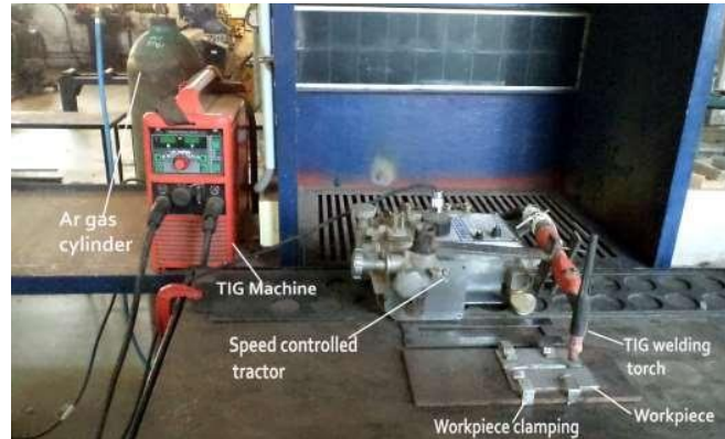
Fig. 3 – Experimental set-up for TIG welding
