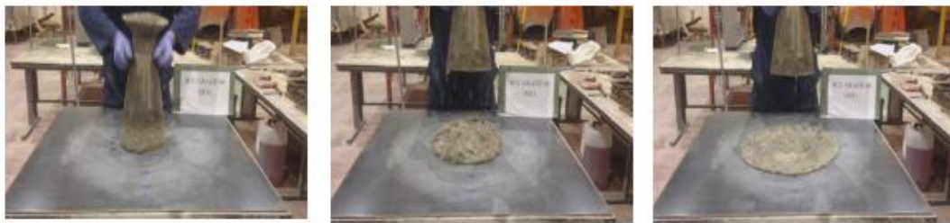
Fig 1 Images captured via video during the slump cone test at each of the three flow phases
